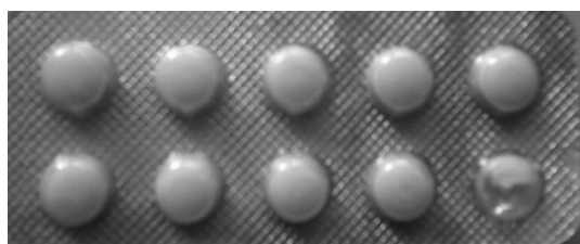
Fig.6: Gray scale image of broken tablet
